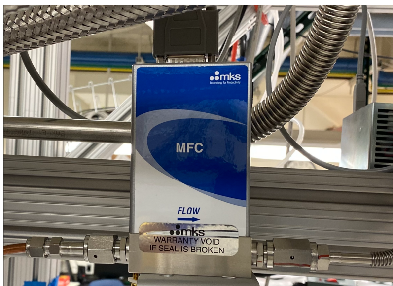
Figure 2.3: The commercial mass flow controller used for our experiment.
