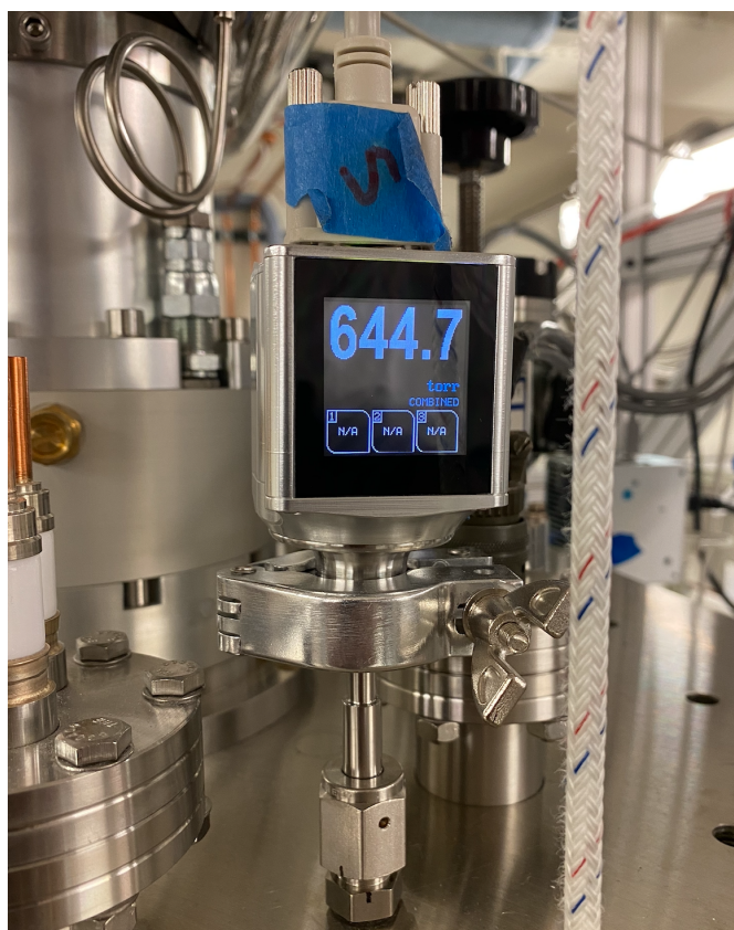
Figure 2.2: The commercial pressure sensor used for our experiment.
