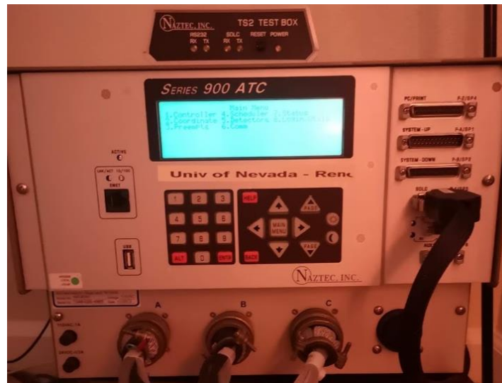
Figure 3. Naztec Series 900 ATC Controller.
