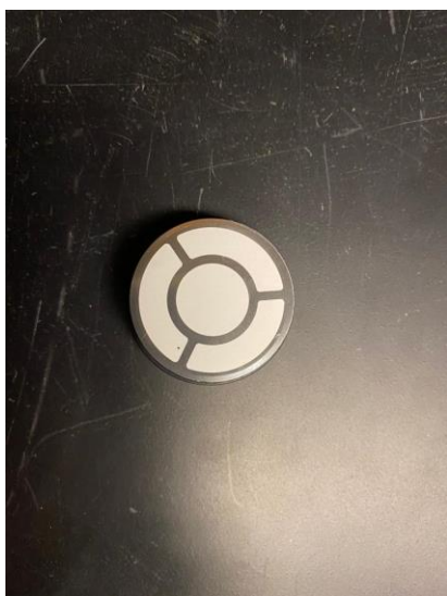
Figure 6: Metal ring and blank filter before sampling.
