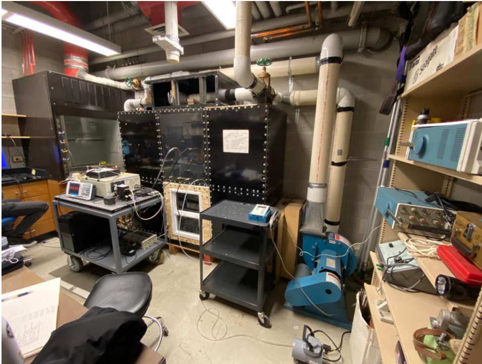
Figure 1: Marple-type dust chamber setup.
