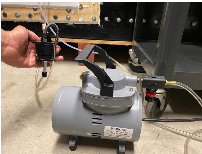
Figure 3: Cyclone sampler arrangement.
