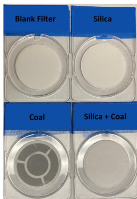
Figure 7: Blank filter and loaded filters obtained from experiments in the aerosol testing chamber.
