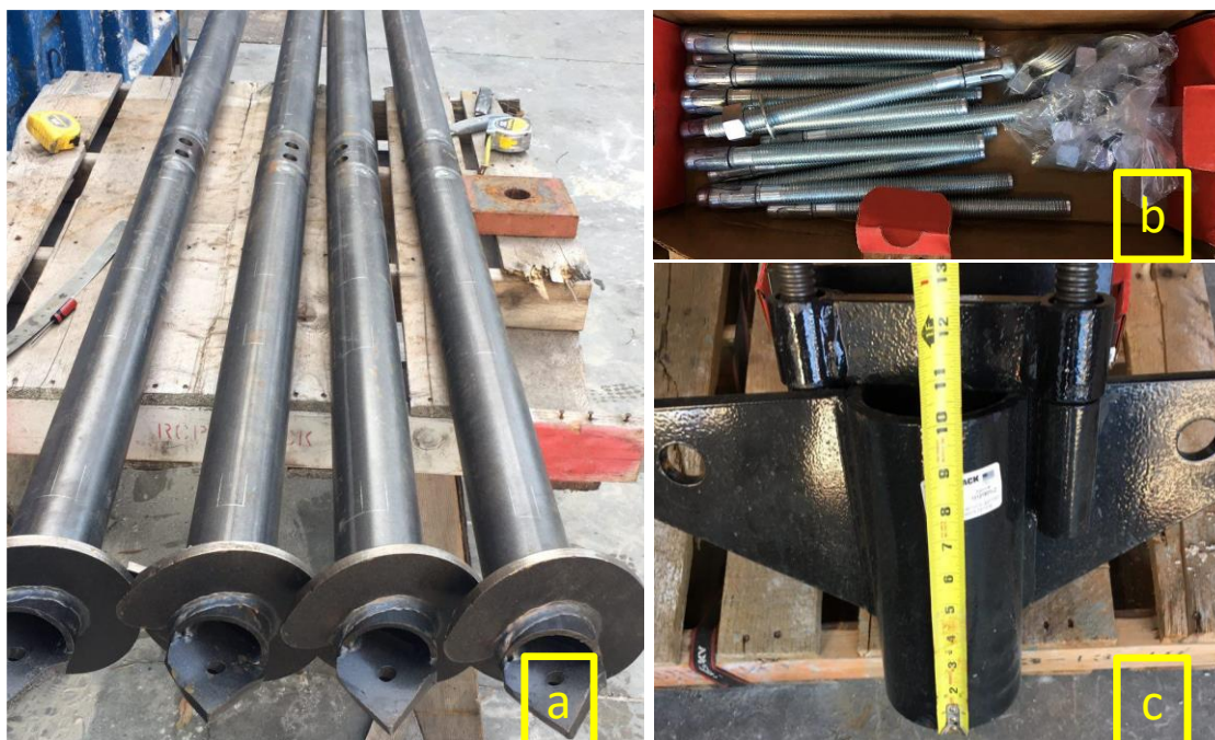
Figure 3.5. Photo of (a) single-helix helical piles (b) bolts and nuts and (c) side bracket
