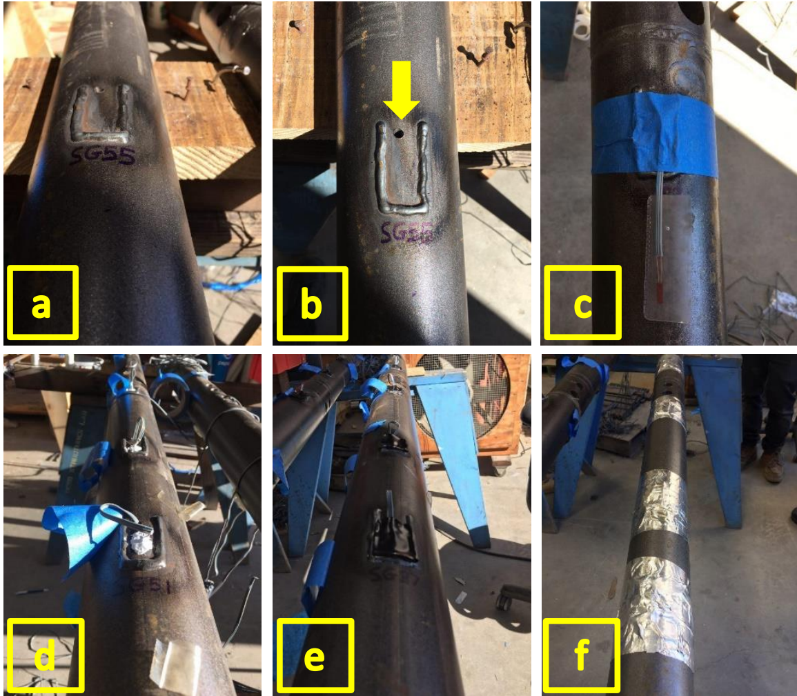
Figure 3.6. Strain gauge installation and protection measures.
