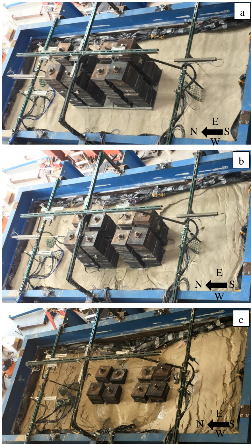
Figure 2.19. Photos of baseline model: (a) before Shake 1-1 (b) after Shake 1-1; and (c) after Shake 1-2.
