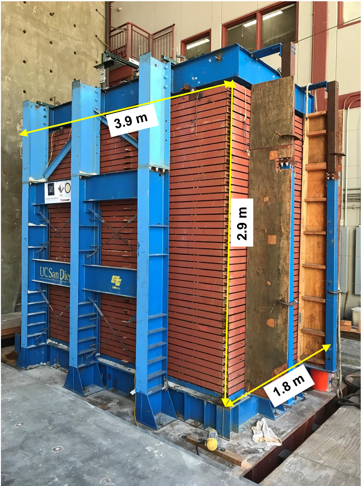
Figure 2.1. Shake table facility and laminar soil box at UC San Diego Powell Laboratory
