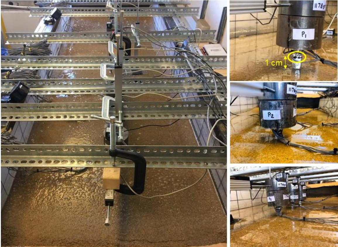
Figure 4.6. Model ground and pile configuration after first shaking in Test #18
