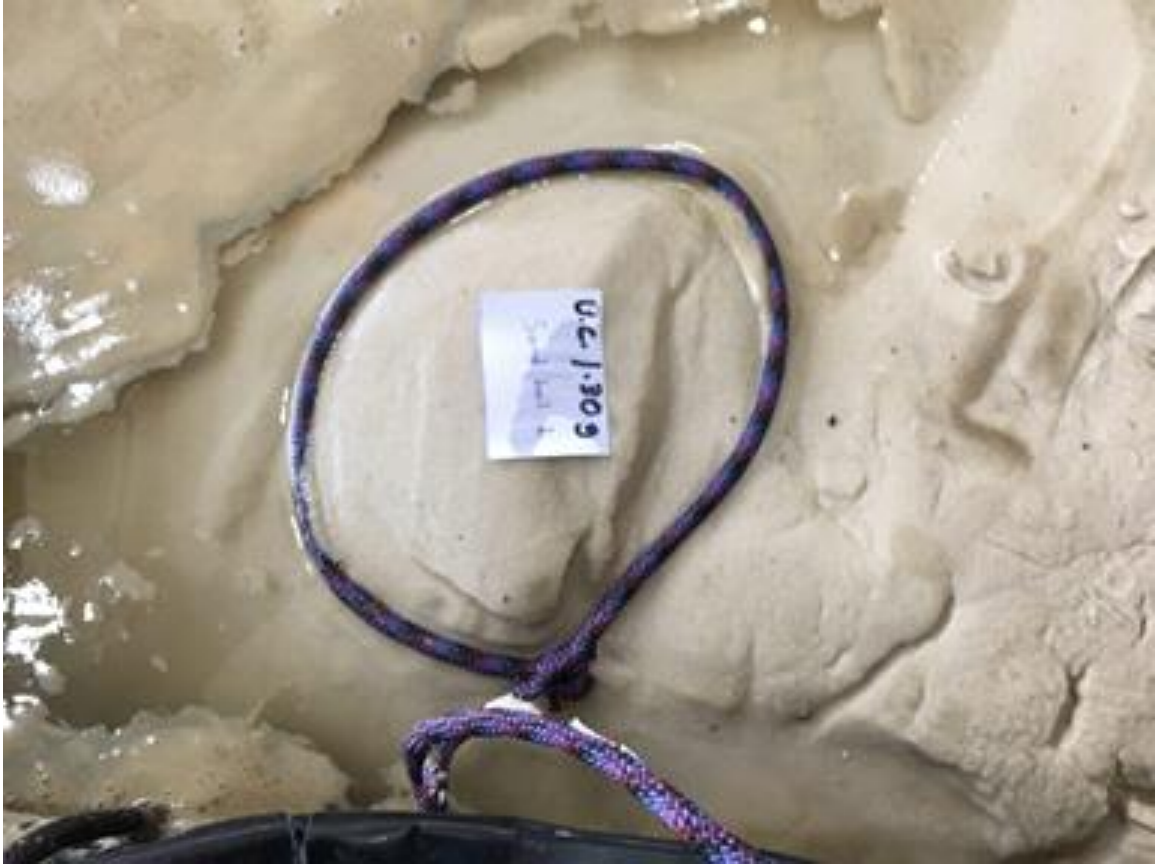
Figure 2.14. Observed sand ejecta after Shake 1-1.
