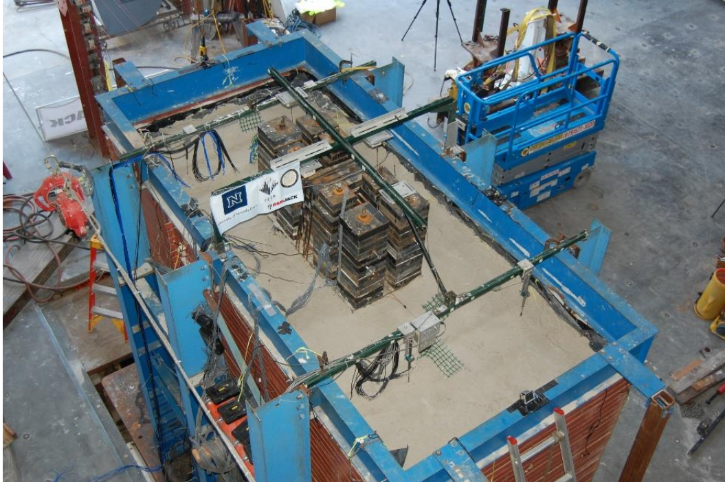
Figure 3.3. Model shallow foundation and superstructure weights in the Helical Pile test.
