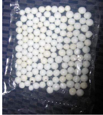
Heat sealed plastic swollen at altitude
