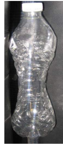
Bottle collapsed at airport
