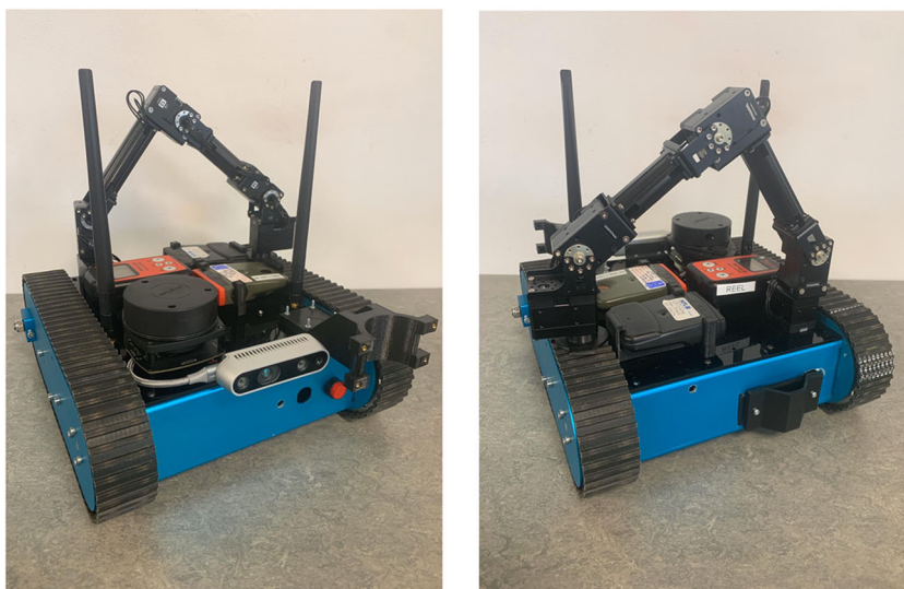
FIGURE 3 Vega, in wireless form with manipulator, ThermoFisher RadEye G10 Gamma sensor, LiDAR and 3D Camera [Color figure can be viewed at wileyonlinelibrary.com ]
