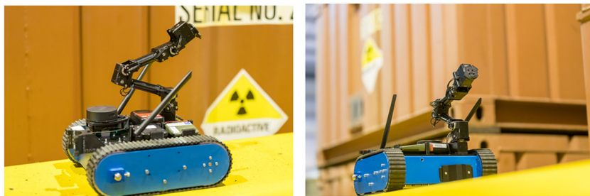
FIGURE 5 Vega with manipulator, during active deployment in the Dounreay waste store [Color figure can be viewed at wileyonlinelibrary.com ]
