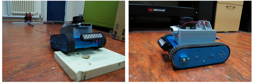
FIGURE 7 Vega, in tethered form with common sensor configuration, LiDAR and 3D Camera, being demonstrated at an inactive test for AWE in the United Kingdom [Color figure can be viewed at wileyonlinelibrary.com ]
