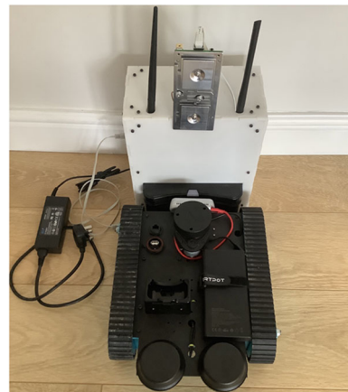
FIGURE 2 Vega docked to base station. Base station features include a directional antenna for a high power router, an omni-directional antenna for a local hot-spot router, and Ethernet connectivity and power supply [Color figure can be viewed at wileyonlinelibrary.com ]
