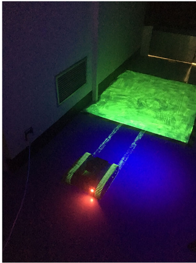
FIGURE 11 Contamination testing using fluorescing rodent tracking powder [Color figure can be viewed at wileyonlinelibrary.com ]
