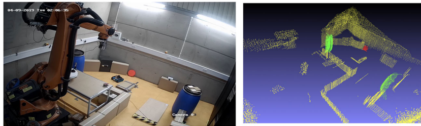
FIGURE 8 Fenswood (University of Bristol) inactive test for AWE. Left image shows Vega positioned beside a gamma source (red disk), with Imitec CC-RIAS mounted as payload. Right image shows an example of the live point cloud produced by the robot, which can be saved and evaluated at the operators discretion. Note the gamma source highlighted in red, and the two barrels highlighted in green [Color figure can be viewed at wileyonlinelibrary.com ]
