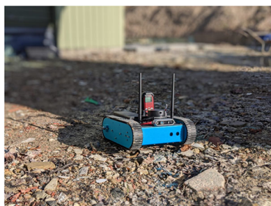
FIGURE 6 Vega, demonstrating locomotion over rough terrain [Color figure can be viewed at wileyonlinelibrary.com ]
