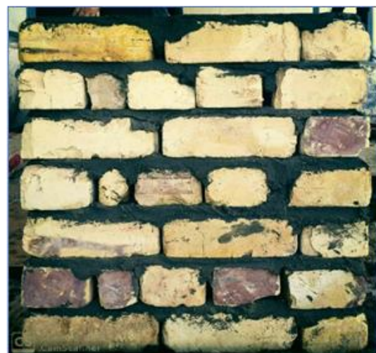
Figure 2. Construction of the masonry wallettes.
