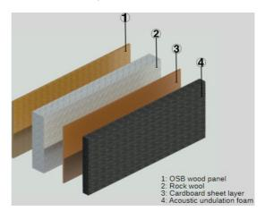
**Figure 2.** Internal layers of the used facility built for sound insertion loss measurement.
