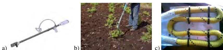
Figure 2. Portable weed spot-control device: a – device model; b – device in operation; c – working element of device.
