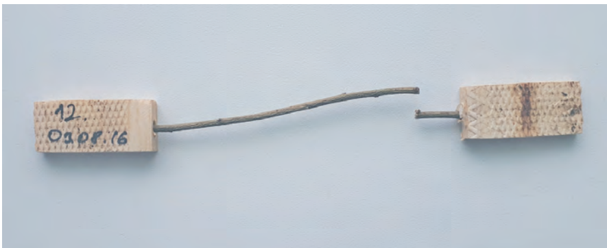
Figure 9. The blueberry plant's stem test unit with clamps at the end of the test.
