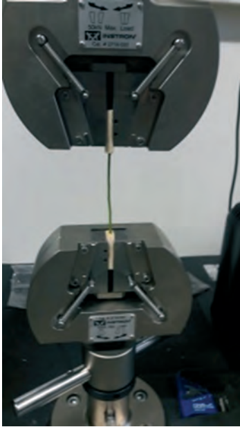
Figure 8. Measuring instrument: INSTRON 5969L2610.
