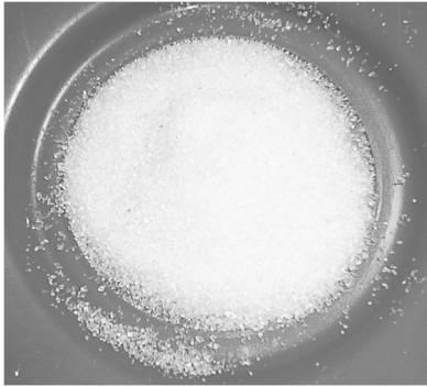
Figure 1. The polymer hydrogel composition in the dried state.
