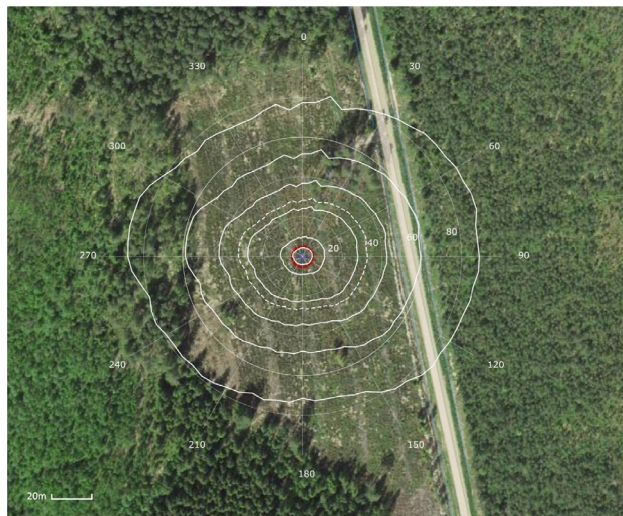
Fig. 1. Footprint area of the study site (using the model by KJjun et al., 2004). Thinner lines and corresponding numbers represent the distances from the tower in metres and direction in degrees from the north. Thick solid lines are the cumulative footprint (1%, 10%, 30%, 50%, 70%, 90%) distances. Dashed line denotes the peak contributing distance. The road in the footprint area has a low traffic load.
