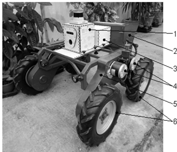
Figure 1. Experimental prototype of an agricultural robot: 1 – sensor bundle; 2 – lithium batteries for lower body; 3 – lithium batteries for sensor bundle; 4 – brushed DC motors; 5 – chassis; 6 – wheels.
