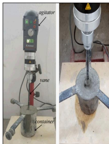
Fig. 8–The components of the rheometer.
