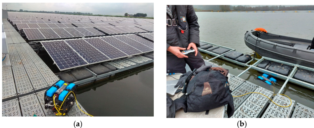
Figure 4. Measurements with the underwater drone/ROV: (a) Impression of the underwater drone equipped with various sensors near the solar panels; (b) operation of the underwater drone from the floating platform to collect depth profiles and inspect the floater blocks.
