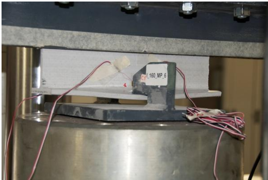
Figure 3.35b. Failure mode of I_160_MP_6 specimen of 300 mm length.
