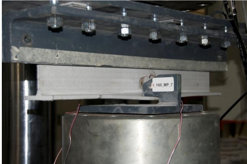
Figure 3.35c. Failure mode of I_160_MP_7 specimen of 600 mm length.
