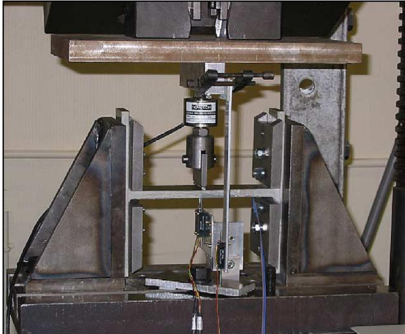
Fig. 1.63. Photograph of the test set up showing the web of a WF specimen with clamped flanges being tested in three-point flexure.
