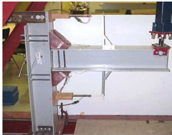
Figure 1.33. Test Setup for Exterior Connections.
