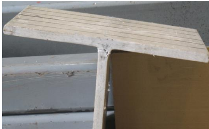
Figure 4.37. Failure of H_8" × 8" × 3/8" (203.2 mm × 203.2 mm × 9.53 mm)_R specimen.
