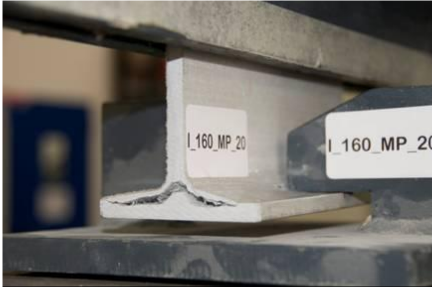
Figure 3.35a. Failure mode of I_160_MP_20 specimen of 200 mm length.
