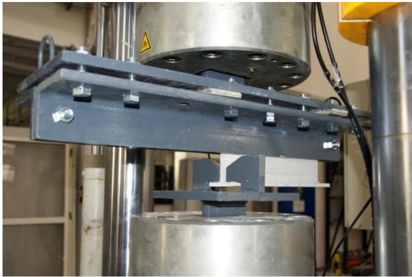
Figure 3.1. End Point Pull-Out Test Setup.
