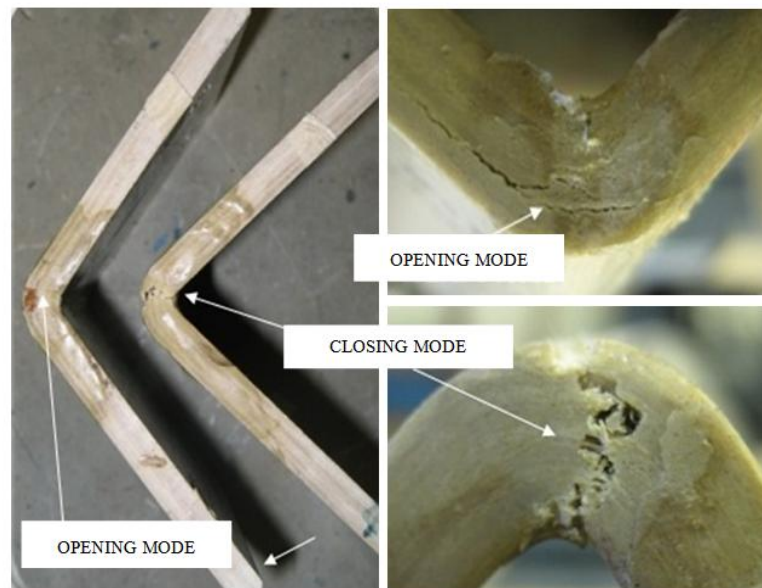
Figure 4.43. Failure of L-profile specimens, opening and closing mode .
