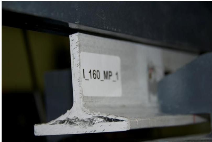
Figure 3.16. Web/Flange Junction Failure of I_160_MP_1 specimen.
