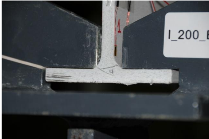
Figure 3.23. Web/Flange Junction Failure of I_200_EP_2 specimen.
