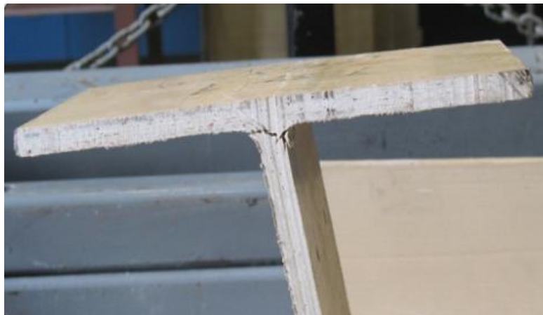
Figure 4.34. Failure of H 10 " × 10" × 1/2" (254 mm × 254 mm × 12.7 mm) _R specimen.
