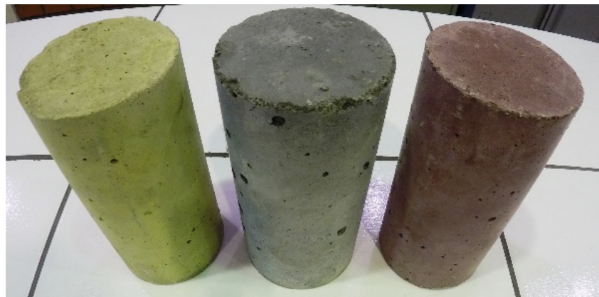
Figure 1. Colored concretes used in the paper: 16 MPa in yellow, 54 MPa in blue, and 85 MPa in red.
