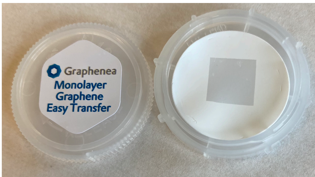
Figure 3.4: 1 cm \times 1 cm easy transfer monolayer graphene from Graphenea on a polymer film.
