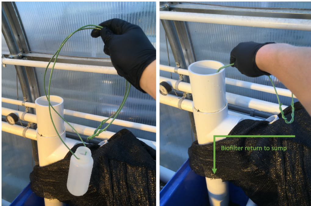
Figure 35. Biofilter effluent collector and sample collection method.
