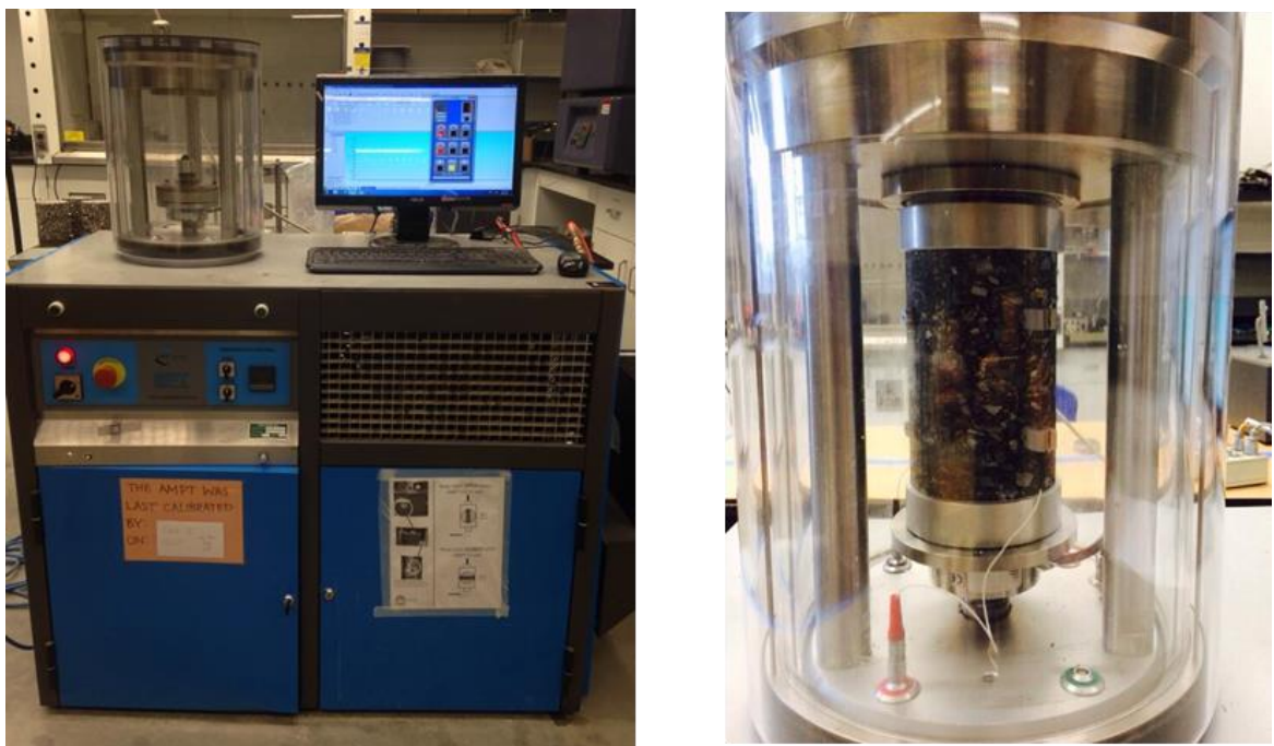
Figure 2-6 AMPT and complex modulus testing configuration
