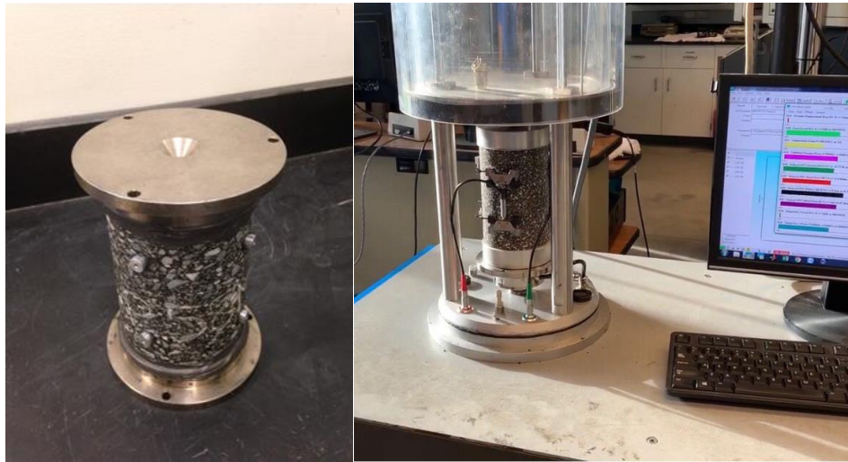
Figure 2-7 Fatigue test specimen and configuration in AMPT
