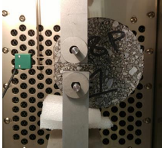
Figure 2-8 DCT test specimen and configuration in UTM
