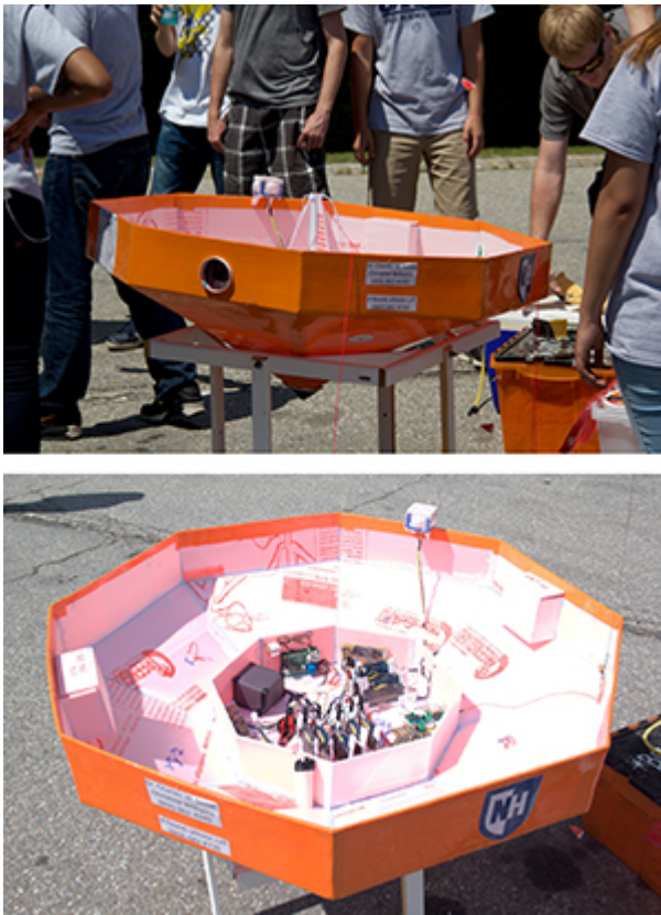
Fig. 3. (top) Film-covered Styrofoam™ payload from the November 2015 launch. A Sun sensor is mounted on the edge of the payload, and the camera port is visible in the side. (bottom) Instruments reside in a “hat box” that provides added stiffness to the design. Credit: UNH
