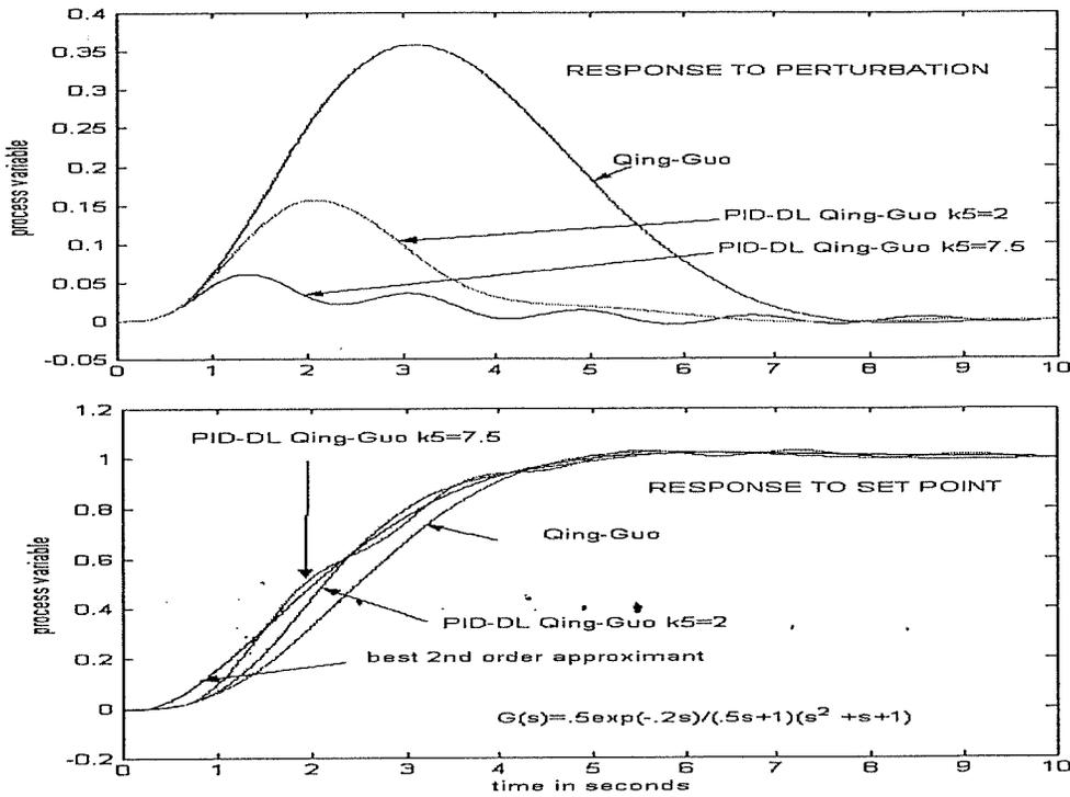
Figure 7: Plant response as a function of outer loop PID gain  $k_5$  (example 2)
