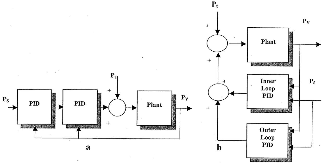
Figure 2: a) A classical 2 degrees of freedom PID; b) A dual loop 2DOF PID
