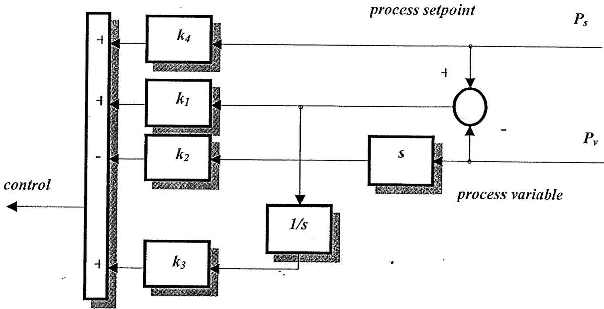
Figure 3: Standard mechanization of an industrial PID
