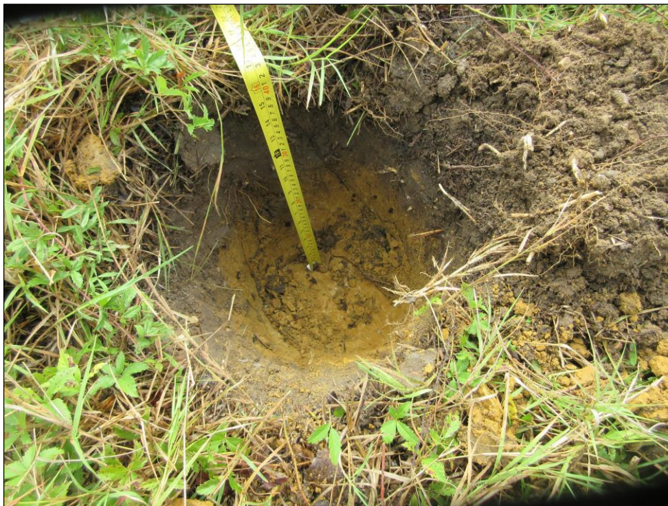
Figure 11: Shovel test at the North launch containing indurated mixed clay at shallow depth; facing down.
