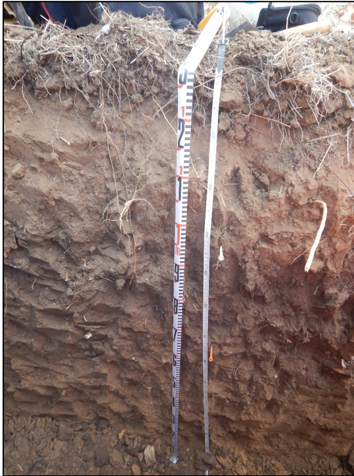
Figure 7. Soil profile of BHT3 showing three strata.
