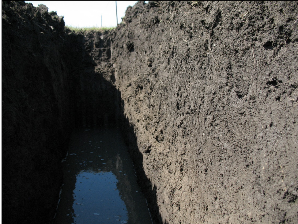
Figure A-8. Overview of water table encountered in Trin05; facing west.
