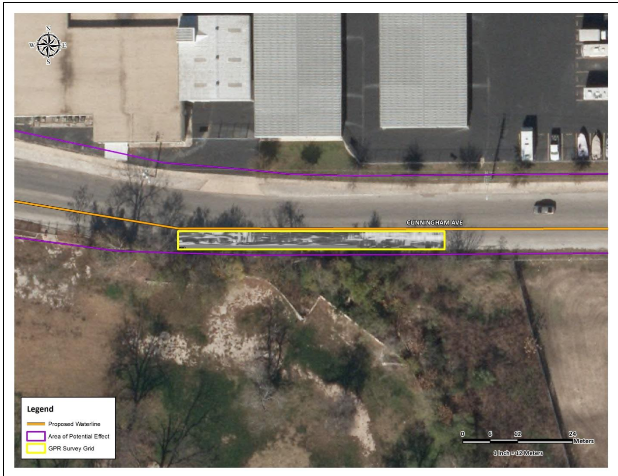
Figure 5-2. The 3-D model of the GPR survey displaying the signal readings at 85 cm below surface.
