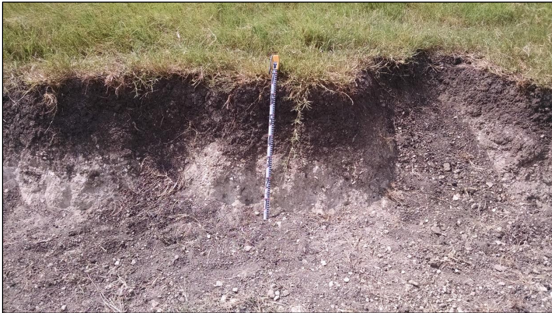
Photo 5. Cut bank in small drainage through center of project area. Note shallow soils above decomposing bedrock. View the south.
