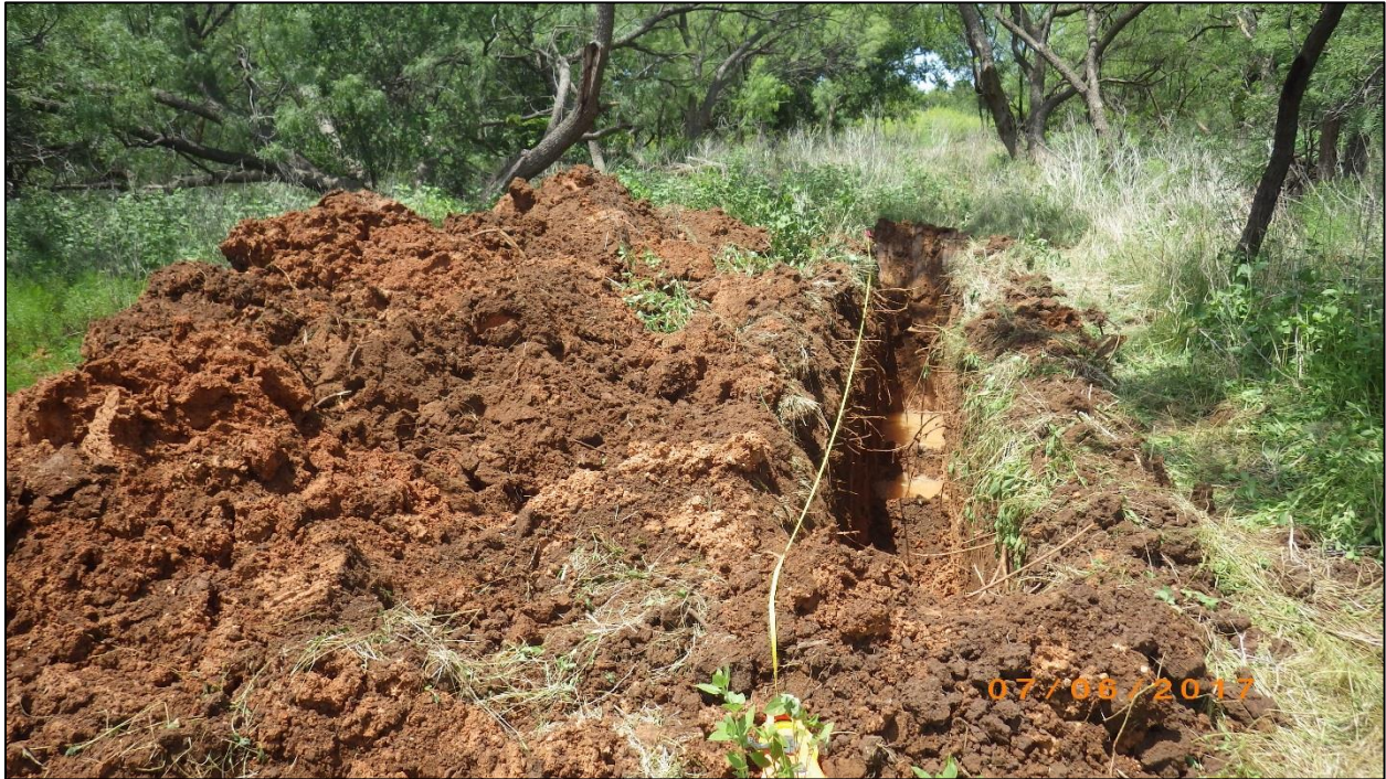
Figure 14. Overview of BHT3 looking north towards wetland. Note water filling in trench.
