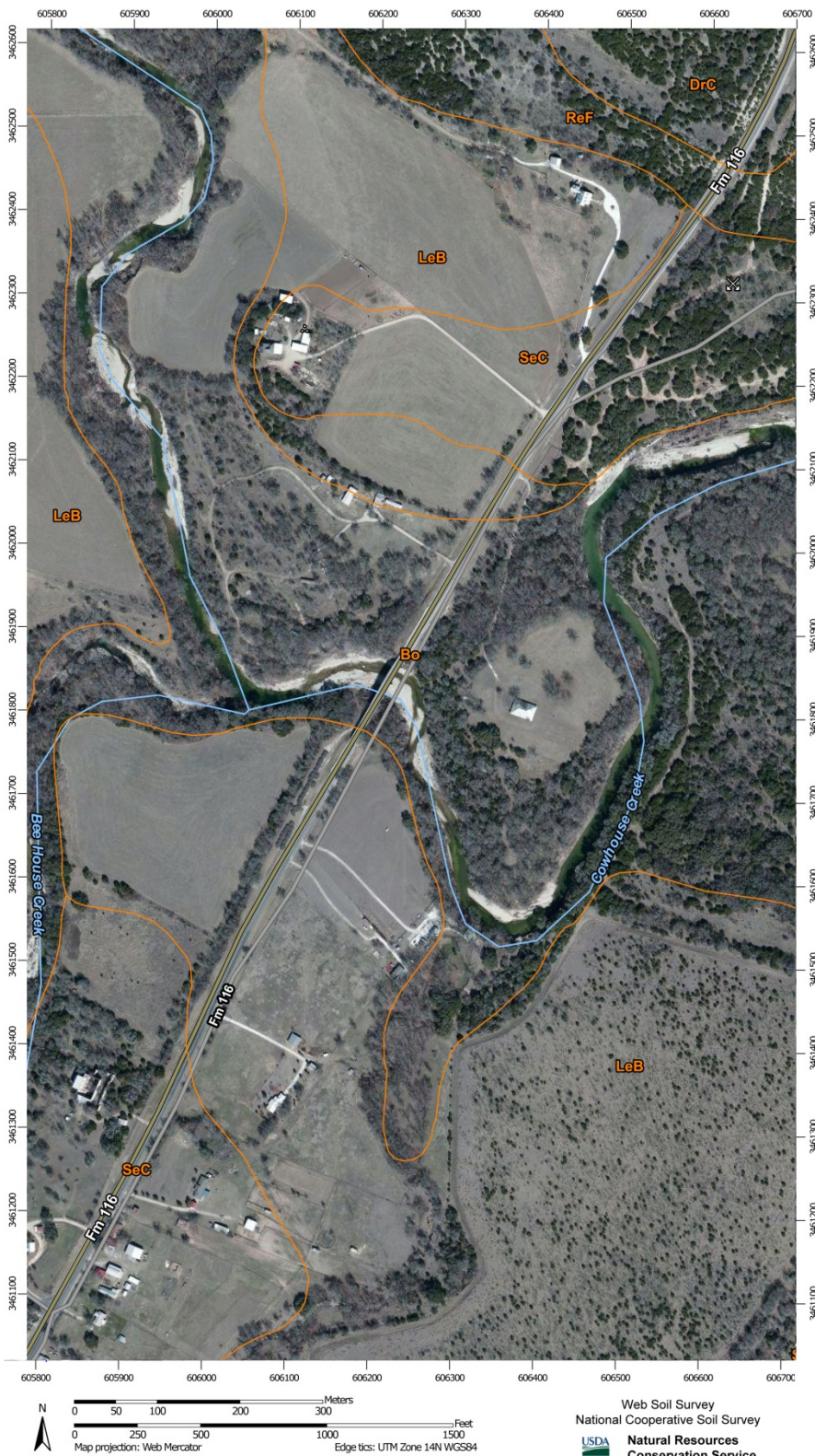
Figure 8: Soil map of study area. Key to mapping units : B0 = Bosque clay loam, 0-1% slopes; DrC = Doss-Real complex, 1-8% slopes; LeB = Lewisville clay loam, 1-3% slopes; ReF = Real-rock outcrop complex, 12-40% slopes; SeC = Seawillow clay loam, 3-5% slopes.
