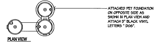
10 SECTION: REMOVABLE BOLLARD Scale: 3/4" = 1'-0"
