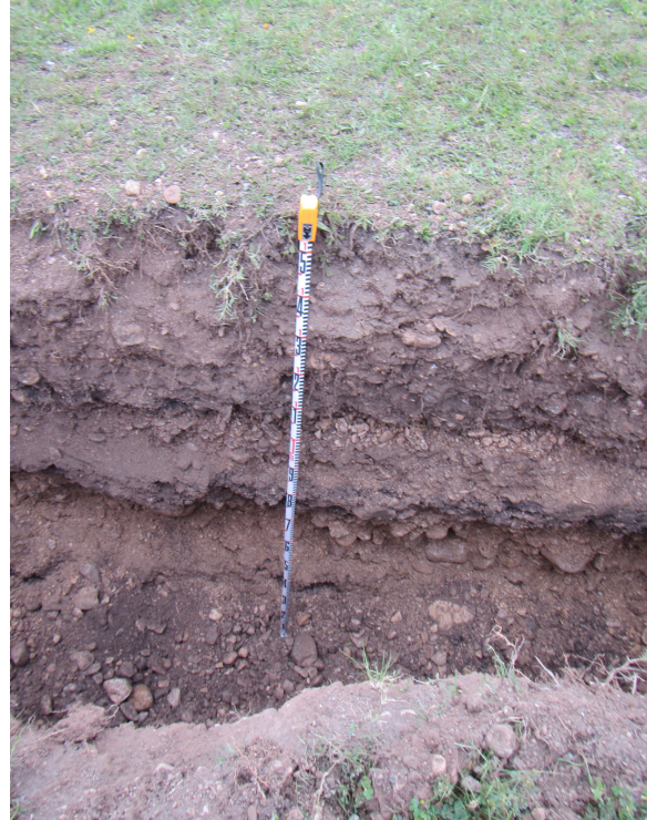
Figure 10. West wall of Trench 2 showing upward-fining sequence of alluvial gravels and sands on the modern Guadalupe River floodplain.
