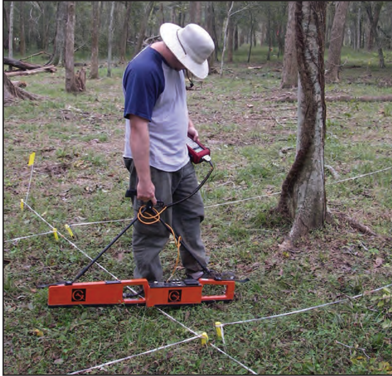
Figure 7-10. Bryan Haley using the Geonics EM38B electromagnetic induction meter within the large cleared area of the south tract.
