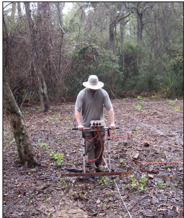
Figure 7-7. The Geoscan RM-15 resistance meter in use in the cleared area in the north tract.
