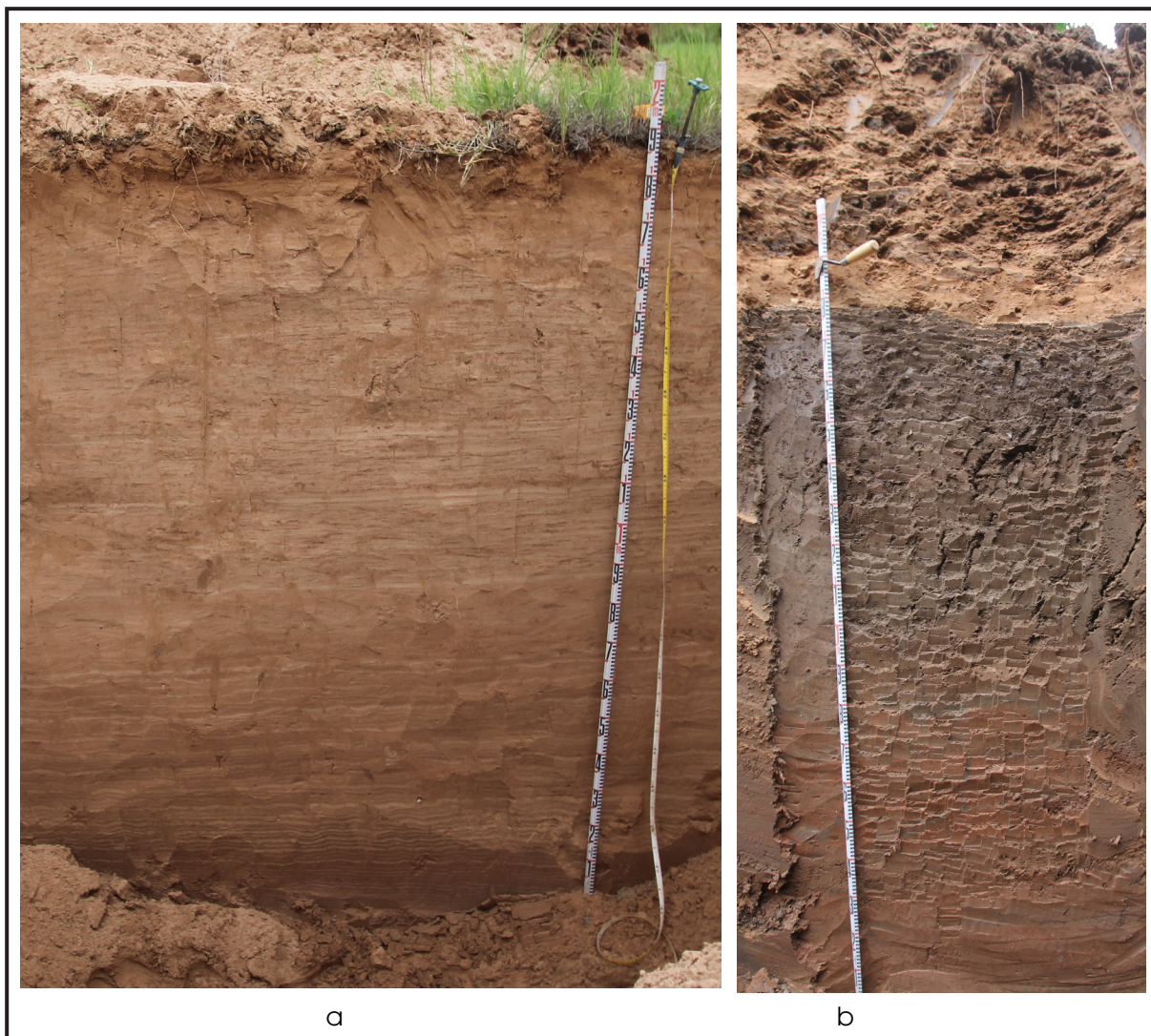
Figure 12. Photographs of Trenches 21 and 33. (a) View of Trench 21 showing a nearly 2-m-thick package of ripple-laminated sand (note the distinct 20–30-cm-thick bed sets that dip gently to the left [north]); (b) view of Trench 33 showing a massive distal flood basin facies shallowly buried beneath 85 cm of introduced earthen fill (note the soil formed in the deposit and the appearance of alternating-colored thin beds of mud below 1 m on the scale).
