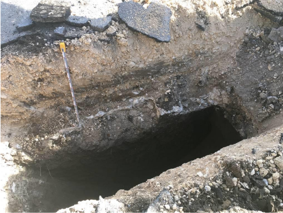
Photo #7: BHT 3 profile exposure with measuring tape/scale resting atop concrete footing.
