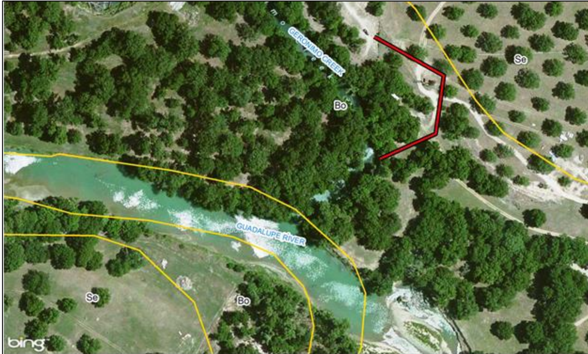
Figure 2-5. Aerial photograph depicting mapped soil units in the area of potential effect immediately east of Geronimo Creek south of Seguin, Texas.
