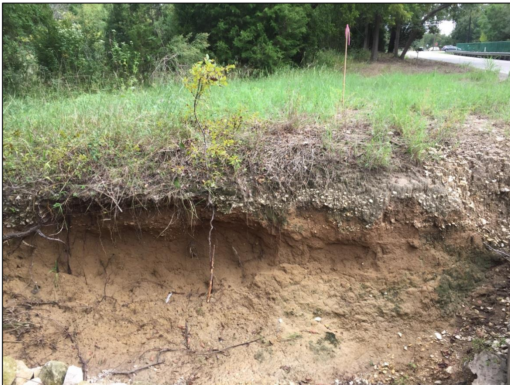
Figure 13. Eroded gully between Hairy Man Road and Brushy Creek, illustrating rubified, calcareous gravelly terrace soils.
