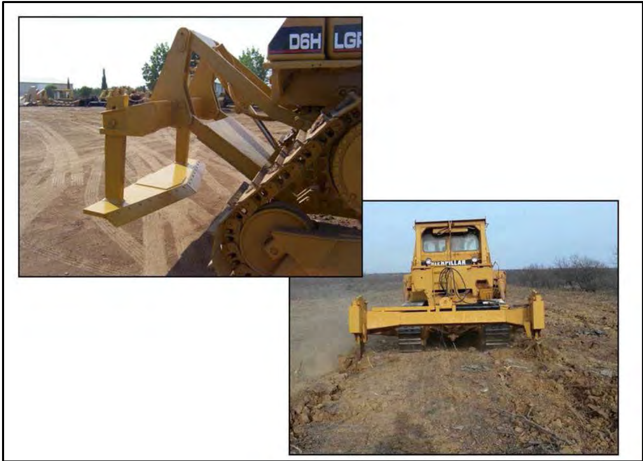
Figure 6.17. Illustrations of root plow equipment, showing the mechanics and impacts of use. Photographs from the internet (top left: http://www.industrialbuckets.com/English/Attachments/RootPlows/RootPlows.html ; bottom right: https://www.youtube.com/watch?v=m-7MboQ6_QM ).
