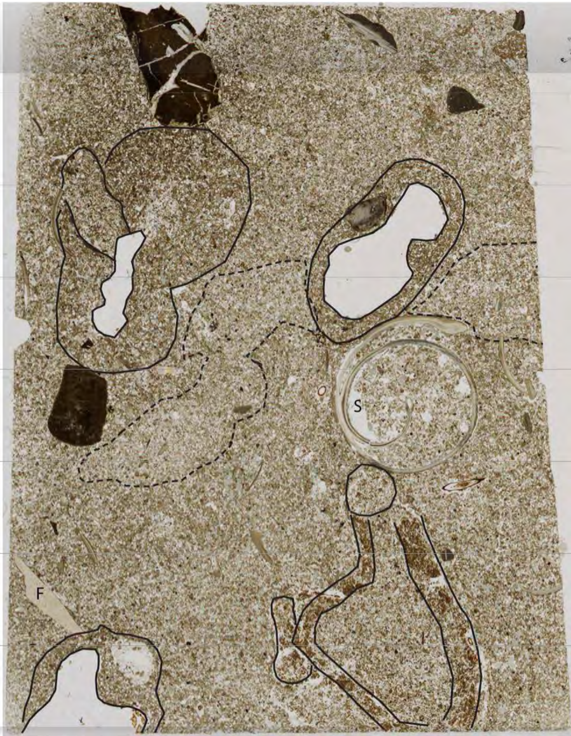
Figure B11: Annotated view of the transmitted light scan of the thin section made from slab 8b of the 45-53 cm block. Most of the features outlined are either open chambers or filled chambers with a relatively thick coat of sediment that is more organic rich and/or finer textured than the surrounding sediment. Also highlighted are other textural/fabric pedofeatures that are associated with faunal activity which exhibit clear edges, internal features that clearly denote them as passages or filled chambers, or areas with less dense matrix that is probably a passage feature (dashed line) but does
