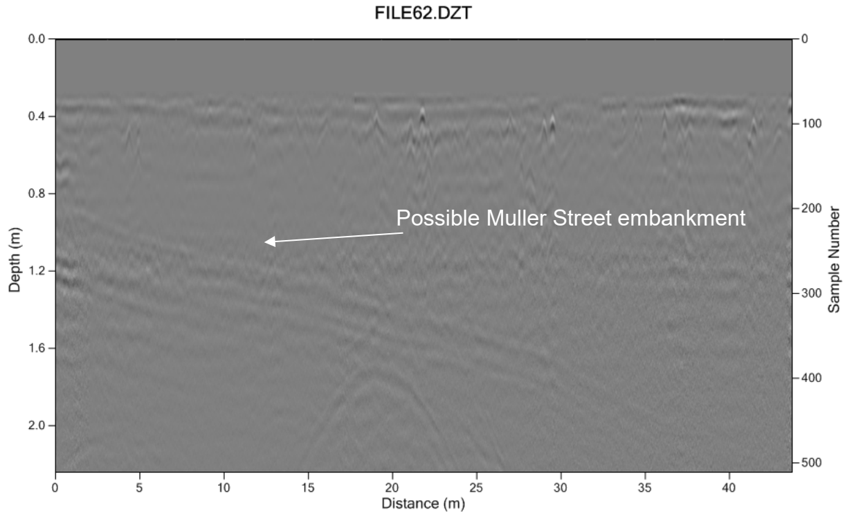
Figure 9: Map of reflection peaks for meter 62. There is a slope starting at 80 cm below the current surface that may indicate the presence of the Muller Street embankment.
