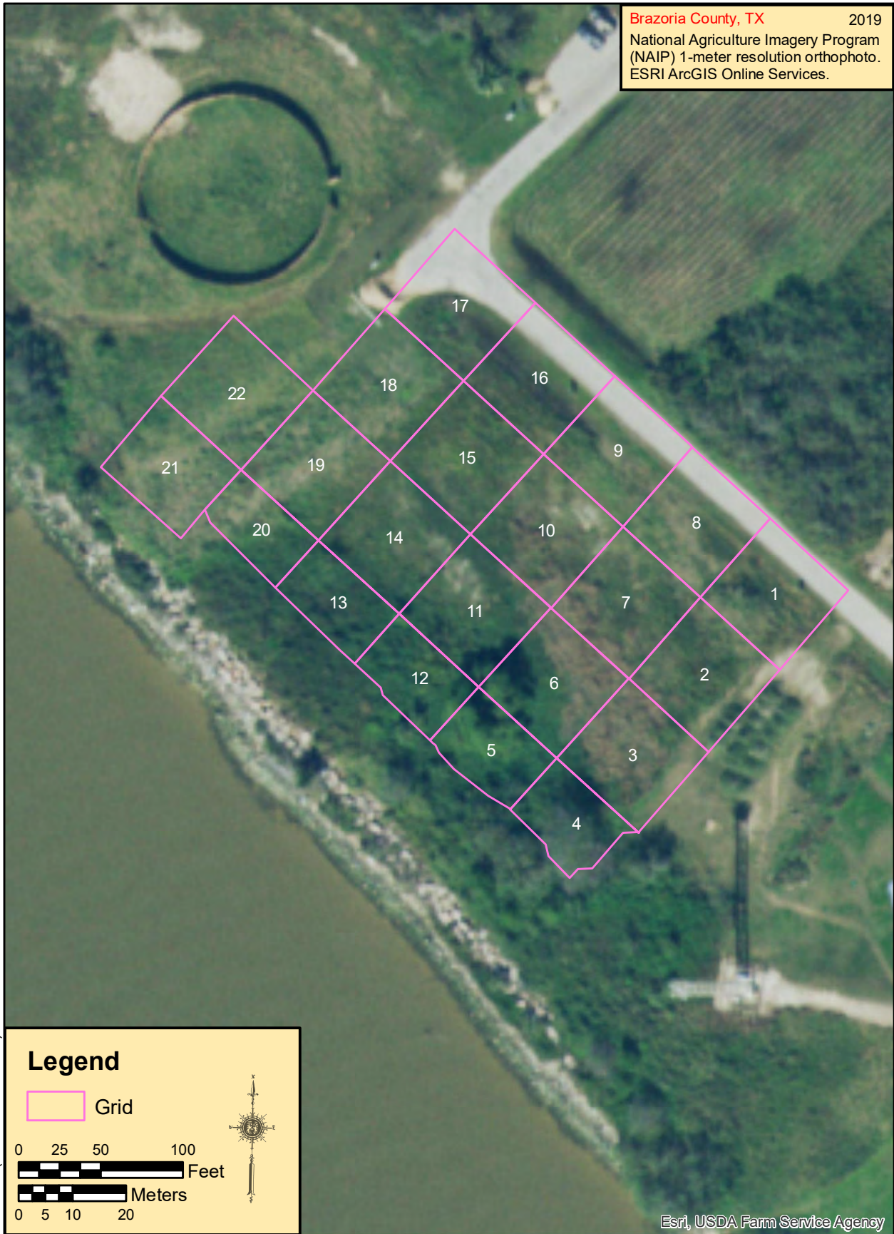
Figure 4.1. Plan view of proposed project area and geophysical survey grids overlaid on aerial imagery.
