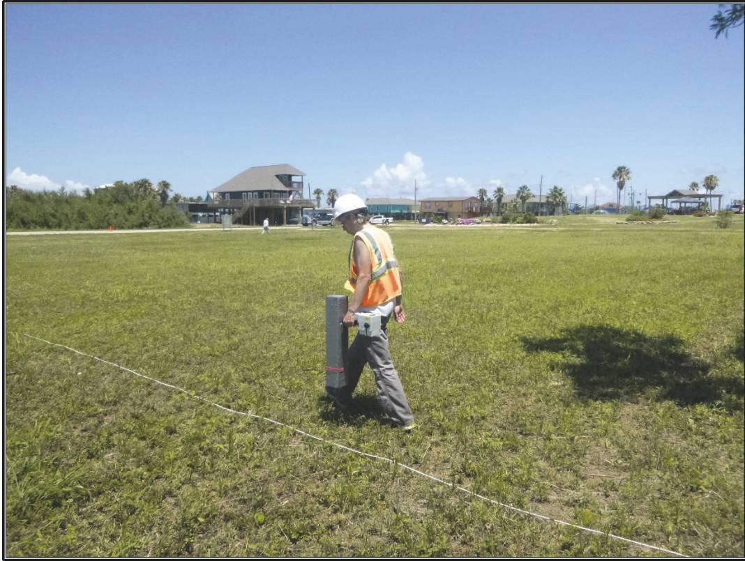
Figure 4.9. Jeremy Pye using the Geoscan FM-256 fluxgate gradiometer during the current geophysical survey, view East (Grid Southeast) in one of the grids in the middle of the field.
