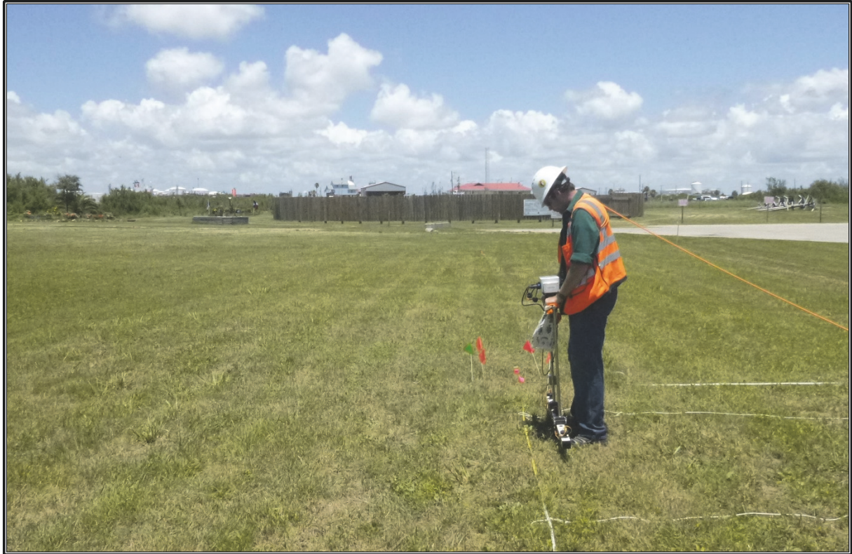
Figure 4.11. Jim Baldwin using the GeoScan RM-85 resistivity meter during the current geophysical survey, view south in one of the grids in the middle of the field.
