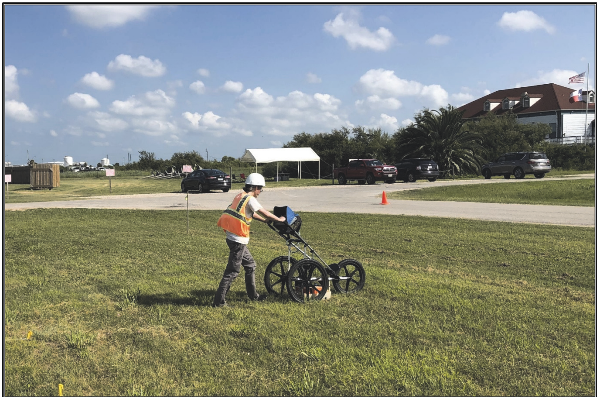
Figure 4.6. Jeremy Pye using the GSSI SIR-3000 GPR, antenna, and survey cart during the current geophysical survey, view north in the northeastern portion of the project area near the intersection of Parkview Road and Monument Avenue.
