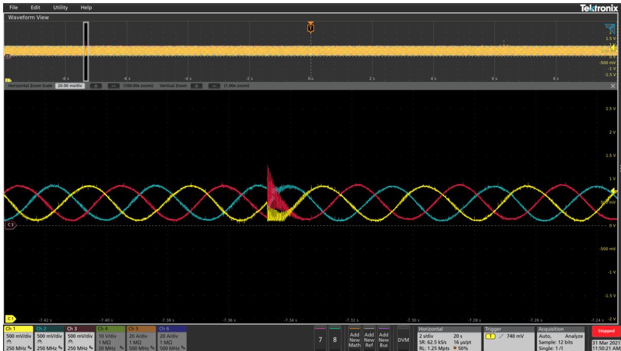
Figure 4.13. Desynchronized 3-phase inverter output waveform during hot-patch
