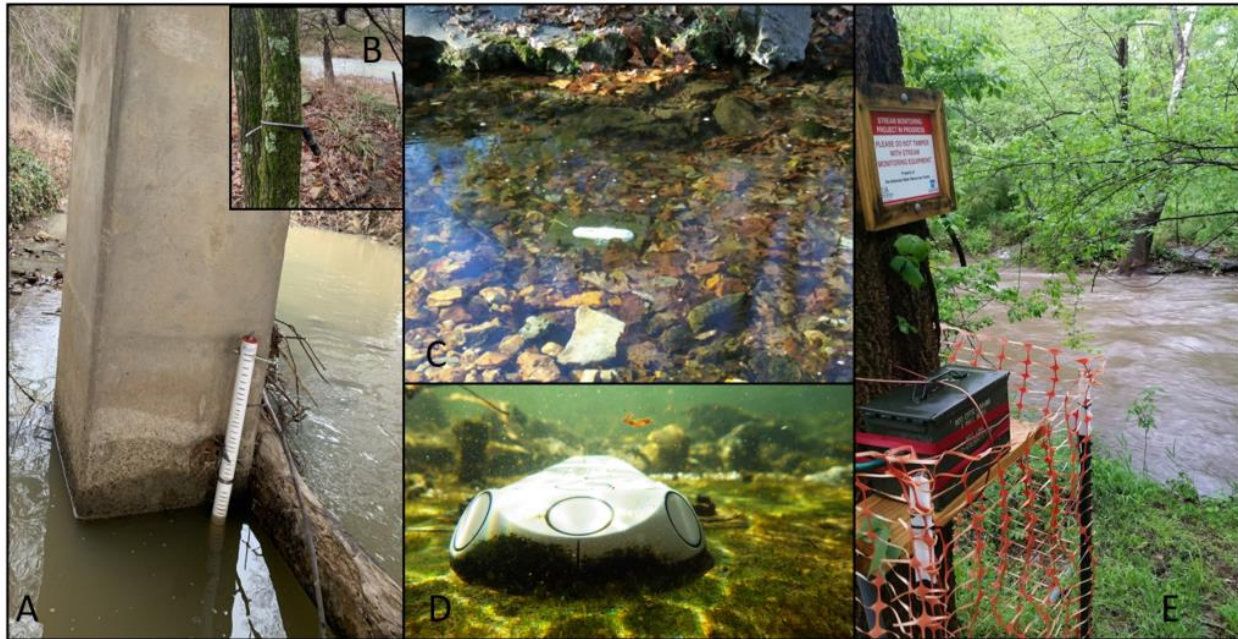
Figure 2: A) Pressure transducer installation on a bridge post, B) atmospheric pressure transducer attached to a tree outside of floodplain, C) SonTek-IQ attached to concrete block in stream channel, D) SonTek-IQ in stream channel, and E) ammo can attached to tree outside of the flood plain to store battery. Photos by B.J. Austin and A.L. Lasater, used with permission.
