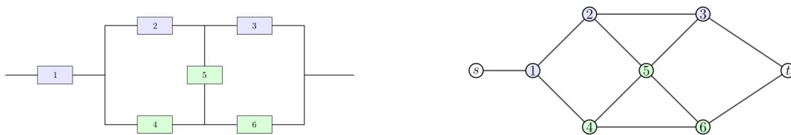
(a) Reliability block diagram of the first system (b) Network representation of validation system used for validation. The network was obtained with nodes s and t appended from the paper by [58].
