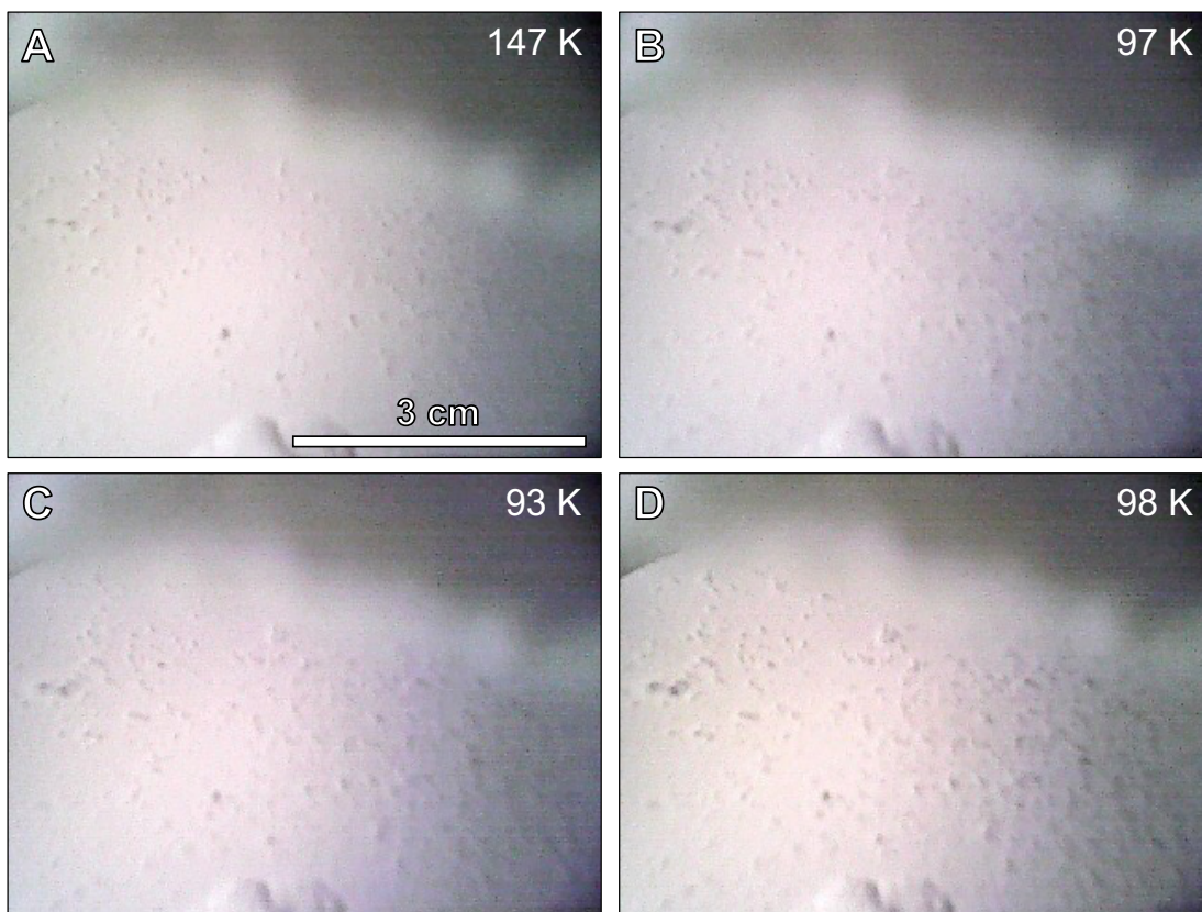
Figure 11. Top-down view of the third C_2H_2 - CH_3CN mixture in the sample dish. Note how the sample morphology maintains consistency even though the temperature was cooled from 147 K to 93 K (A)-(C). We observe an increase in solid particles on the dish from (A) to (D).
