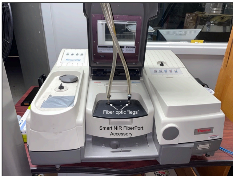
Figure 8. Nicolet 6700 FTIR located below the Titan chamber. Fiber optic “legs” connected to the top of the Smart NIR FiberPort accessory (middle of spectrometer) extend through the chamber with the single terminator end resting just above the sample dish.
