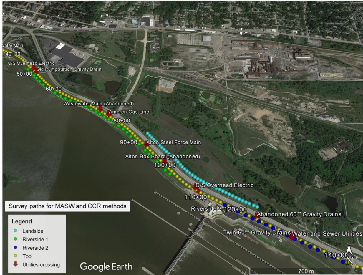
Figure 5.4. Survey paths for MASW and CCR at Melvin Price Reach of the Wood River Levee (Both MASW and CCR were performed along the same paths)
