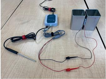
6. Collect temperature and voltage until the ice melts in the ice water. Be sure to stir the water in each beaker regularly to maintain uniform temperatures.
