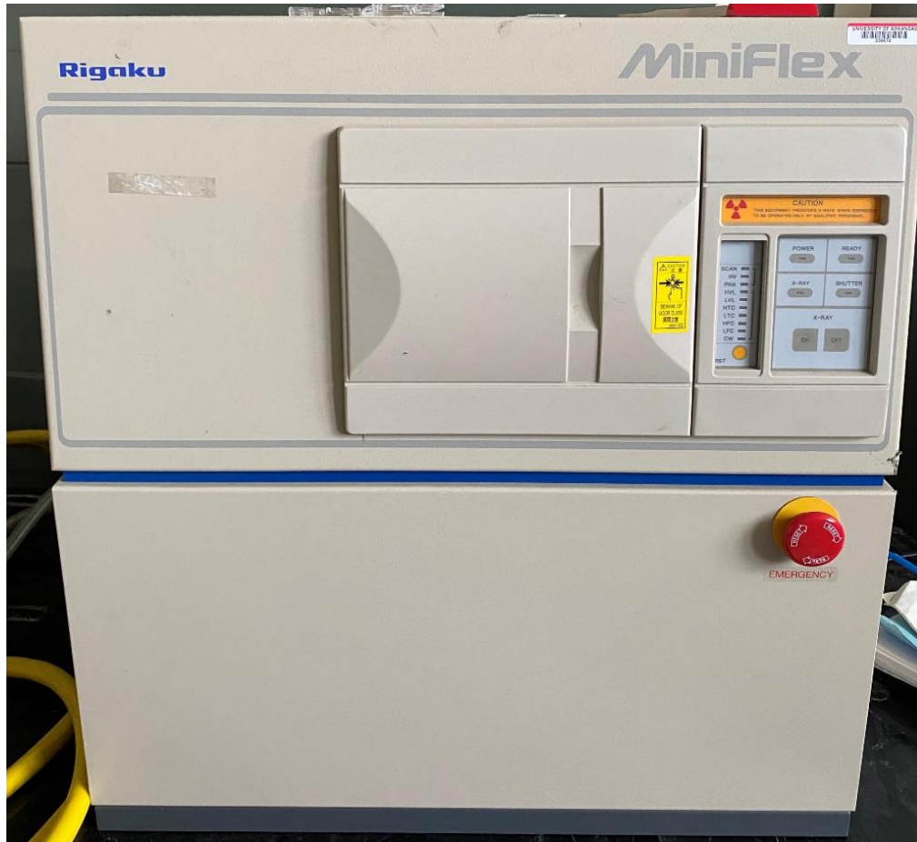
Figure 3.5. Rigaku Miniflex X-ray diffractometer was used to measure the XRD patterns of the synthesized materials. “Photo by Tanveer Ahmed Siddique”
