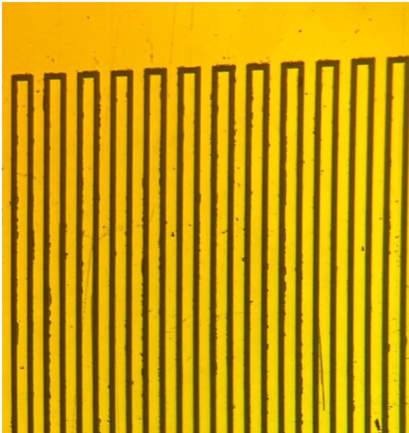
Figure 2.6. The microscopic view of the fabricated device is displaying 10µm interdigital pattern on the samples after lift-off process. “Photo by Tanveer Ahmed Siddique”
