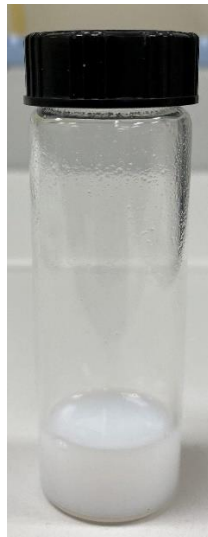
Figure. 2.3. ZnO nanoparticles were dispersed in Butanol for experimental use. “Photo by Tanveer Ahmed Siddique”
