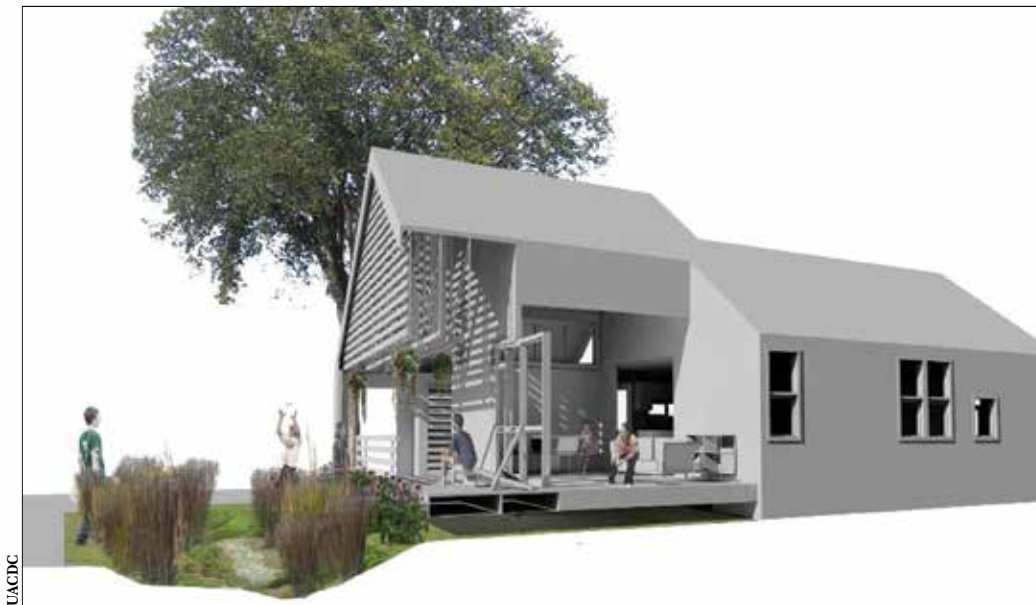
Habitat Trails includes architectural and landscape-design features that promote community and encourage social exchange. This image shows a bioswale in front of the home. Bioswales are infiltration systems that allow rainwater to percolate into the underlying soil.
