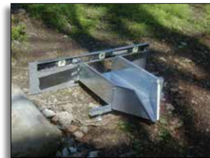
Researchers use a weir (above) to aid in measuring water discharge. Van Brahana, top center, installs a weir at Tree Seep. Jozef Laincz, doctoral student in environmental dynamics, far right, measures water quality as it comes from the seep. Doctoral student Tiong Ee Ting, near right, introduces E. coli into ground water through a barrel, as Ralph Davis and Greg Thoma observe.
