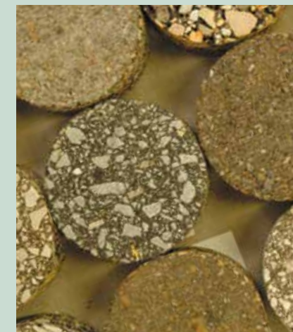
CTTP director Frances Griffith demonstrates a new, more accurate method of density analysis with an asphalt core sealed with the Corelok® vacuum system. Density correlates with asphalt strength: too dense and it ruts easily, not dense enough and it breaks down too fast. As the cores at left show, asphalt composition and density vary greatly, depending on the application.
