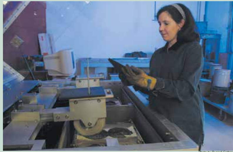
Stacy Williams loads weights onto the track arm of ERSA. Developed through research funded by Mack-Blackwell, ERSA allows asphalt samples to be tested under varying simulated traffic and weather conditions.
