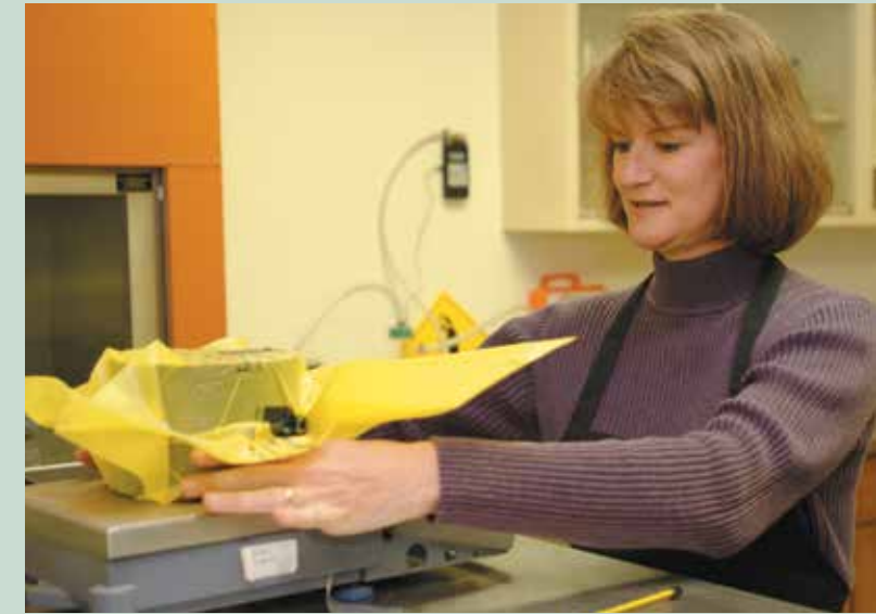
CTTP director Frances Griffith demonstrates a new, more accurate method of density analysis with an asphalt core sealed with the Corelok® vacuum system. Density correlates with asphalt strength: too dense and it ruts easily, not dense enough and it breaks down too fast. As the cores at left show, asphalt composition and density vary greatly, depending on the application.
