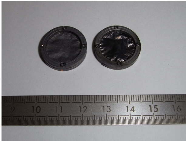
FIG. 3. (Color online). Platinum foil samples blackened by carbon spray (left) and vacuum evaporation (right).
