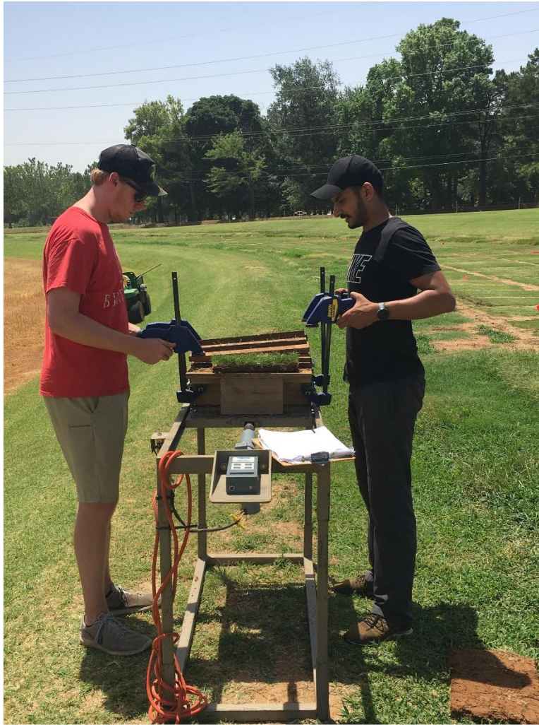
Figure 1. Sod tensile strength testing device.
