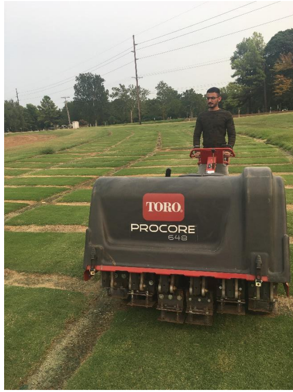
Figure 1. Baldree traffic simulator constructed by modifying Toro ProCore 648 aerification unit
