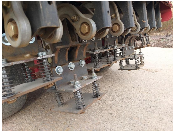
Figure 2. Spring-loaded metal plate feet in place of coring heads.
