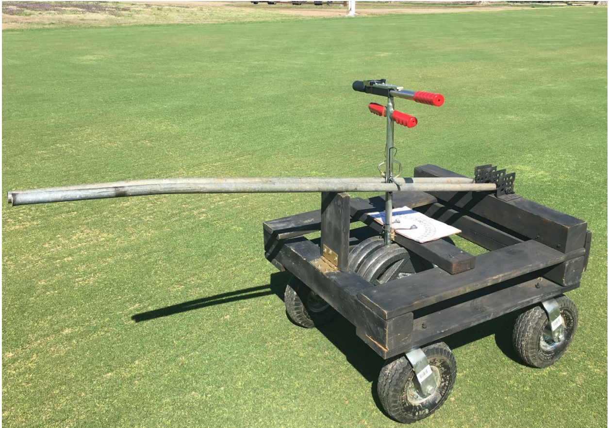
Figure 1. Modified Turf-Tec shear tester
