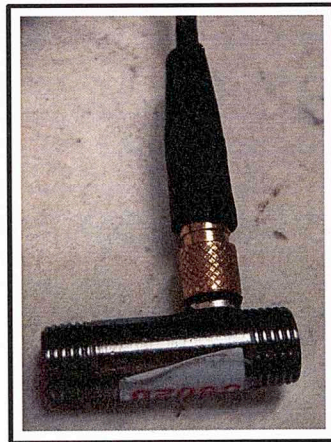
Figure 4.5. Broadband AE transducer. B1025 manufactured by Digital Wave Corporation.
