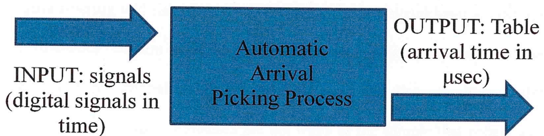
Figure 1.4 Input - output block diagram representation of the automatic picking process to extract the arrival time of a signal or group of signals.
